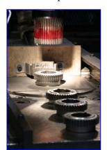
iron-based, powdered alloy. Additions such as chrome, nickel, molebdenum and graphite are added for strength, ductility, and wear resistance. The powder blends are compressed to
